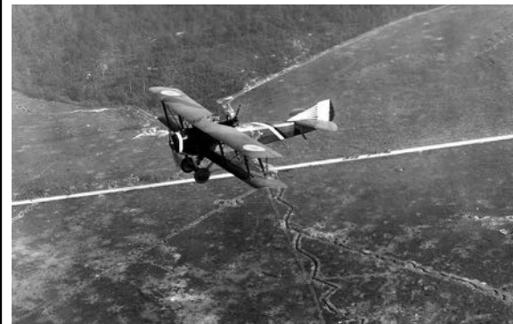
Figure 2 - A French SPAD S.XVI two-seat biplane reconnaissance aircraft, flying over Compiègne Sector, France ca. 1918. Note the zig-zag patterns of defensive trenches in the fields below. Photo courtesy of the San Diego Air and Space Museum Archive.
