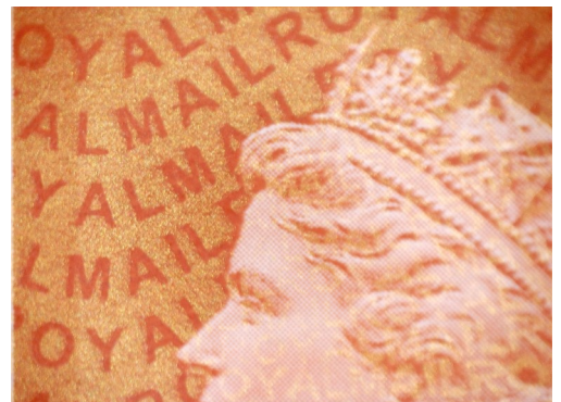
Fig. 11. A trial security overprint using Iriodin® ink.
